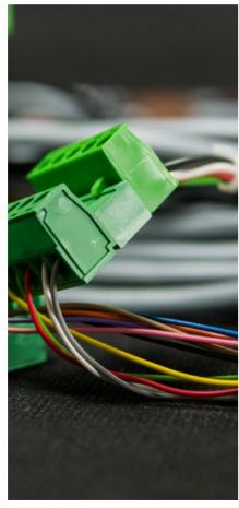
On request, the controllers are supplied both with electric lines and push-buttons terminal boards for floors and car, ready to be placed on jobsite.
